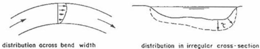
Figure 3. Boundary shear stress in uniform flow (COE 1994).
